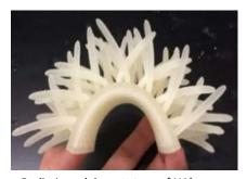
Preliminary lab prototype of UA's impact protection technology, which mimics hedgehog spines
